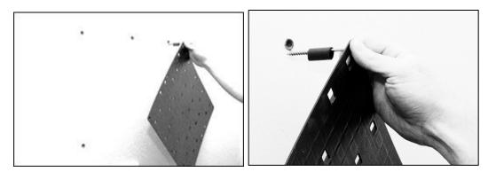
Step 5. Fasten with a star point screwdriver
