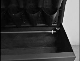
Step 34. Connect the T-full flow connector in the middle of the water tank, pointing the T downwards. Connect the final piece of pipe to the pump
