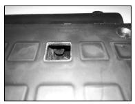
Use a piece of wire and clear the blockage in the nozzle, through the hole in the panel. Below is a picture of what the nozzle looks like, and how deep the wire needs to go to unclog the nozzle
